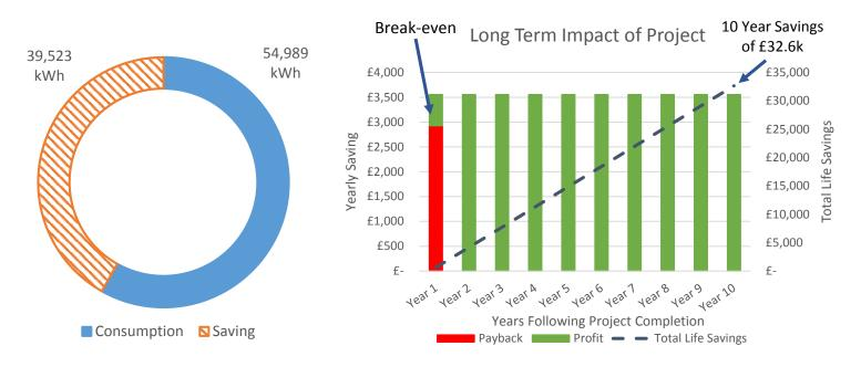
This level of performance significantly exceeded expectations in advance of its installation. The VSD was found to produce savings that were 31% greater than had originally been predicted, with these increased savings also reducing the payback period from just over a year to just under 10 months.
